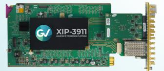
Dual-channel 4K UHD Gearbox IP Application for XIP-3911 and XIP-3901
