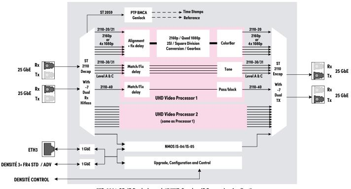
XIP-3901-GB-IP Dual-channel 4K UHD Gearbox IP Processing Application
