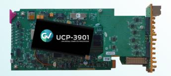
The UCP-3901 is a user-configurable multichannel video/audio-over-IP transceiver developed for use within low-latency and high-bandwidth Ethernet IP networks. The UCP-3901 provides a hardware platform which can offer different functionality depending on the software option loaded. These options are known as *Software-Defined Cores* (SDCs), and can be purchased through a licensing mechanism and loaded as operational needs demand.
