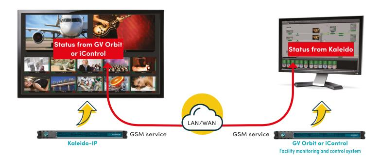
GV Orbit's or iControl's extensive library of third-party devices allows Kaleido-IP to leverage existing IP and MPEG probing devices to increase alarming capabilities.
